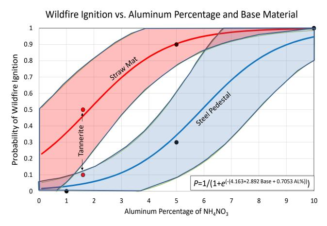
**Figure 9**—Logistic regression model and 95-percent confidence intervals from the 2018 tests relating the probability of wildfire ignition to the aluminum (AL) percentage of the aluminum-ammonium nitrate mass and the base material supporting the exploding target. Data points are averages of the 2018 data for these combinations. Logistic model uses predictors of base = 0 for pedestal and 1 for straw. Model had residual deviance of 40.31 and Akaike Information Criterion of 46.31.
