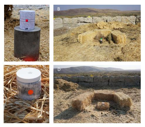
Figure 2—Photographs of target base material used in field tests: (A) close-up view of steel pedestal in 2015 tests, (B) pedestal in 2018, (C) close-up view of straw mat in 2018, and (D) straw mat in 2018.
