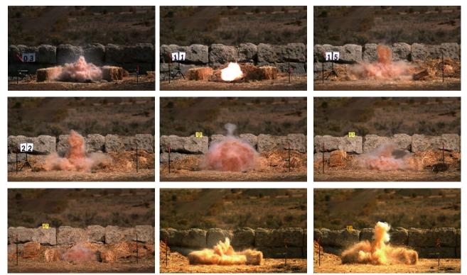
**Figure 12**—Frames from selected 2018 tests showing smaller explosion envelope with little visible burning within the blast volume or burning aluminum particles. Number seen in the photograph is the test number corresponding to those in Appendix 2.
