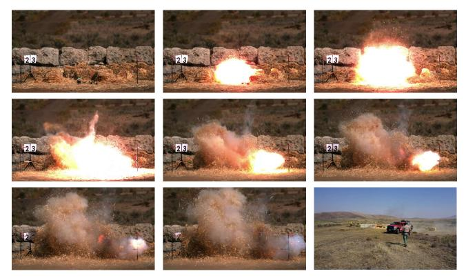
**Figure** 7—Test 23, 2018, 10 percent aluminum, partially mixed. Series showing explosion, vertical and lateral ejection of burning aluminum, residual combustion within the blast zone, and ignition of straw bales.
