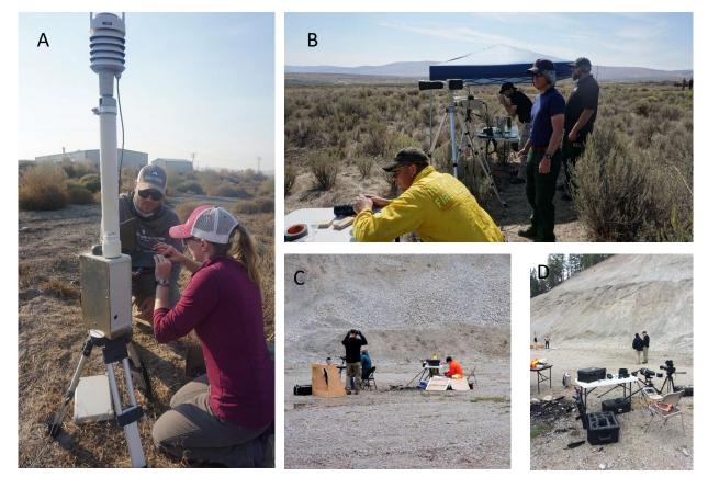
Figure 5—Photographs of (A) portable weather station used in 2018, (B) video cameras behind the firing line in 2018, (C) location of video cameras behind the firing line in 2015, and (D) close-up of video cameras in 2015.
