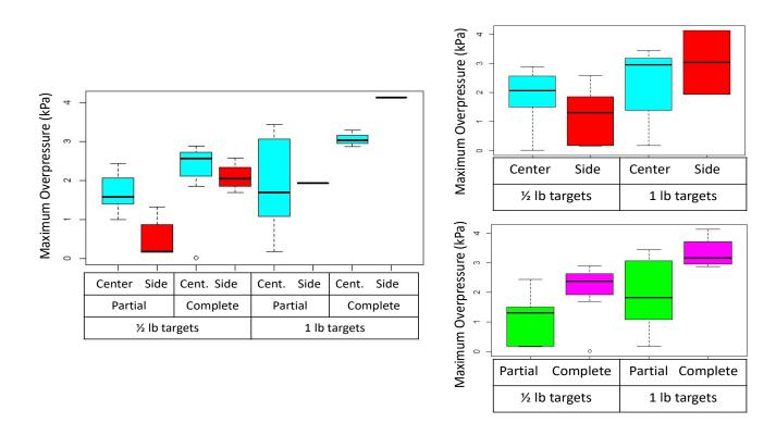
**Figure 16**—Data from 2015 tests showing maximum overpressure (recorded by probe 1; see figure 14) as a function of target size (0.5 lb or 1 lb), completeness of mixing, and bullet placement (side of target vs. center of target). Bullet placement was recorded by high speed video (see figures 7 and 8).
