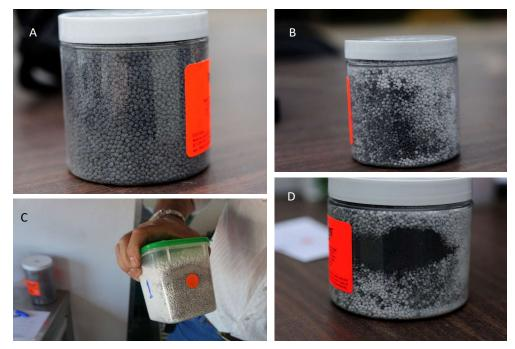
**Figure 4**—Example of (A) complete mixing of aluminum with ammonium nitrate in exploding target compared to the variability of (B) incomplete mixing (Tannerite 0.5-lb target), (C) incomplete mixing of custom target (2018), and (D) incomplete mixing (Tannerite 1-lb target). Localized concentrations of aluminum are clearly visible in the partially mixed targets.
