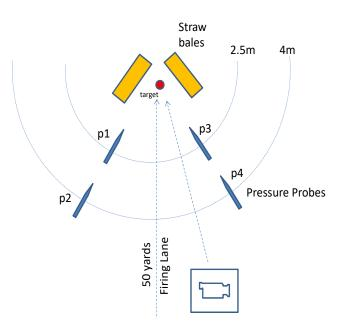
**Figure 1**—Schematic plan for field testing, showing the relative positions of target location, straw bales, pressure probes (P1–P4), and firing lane, and camera locations.
