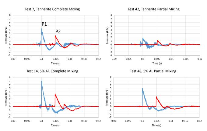
**Figure 14**—Graphs of air pressure perturbation from selected 2018 tests of exploding targets. All targets are 1 lb. Probe 1 (P1, blue) was 8 ft from the target. Probe 2 (P2, red) was 15 ft from the target (see also figure 1). Higher overpressure occurred with additional aluminum. Partial mixing diminished peak overpressure compared to complete mixing.
