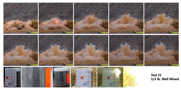
**Figure 13**—Sequence of images from test 51, 2015, showing side impact on well-mixed 0.5-lb target and minimal amounts of glowing material in the explosion envelope.
