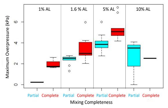
**Figure 15**—Data on maximum overpressure recorded by probe 1 (see figure 14) in 2018 tests showing variation explained by the completeness of target mixing as well as percentage of aluminum (expressed as percentage of ammonium nitrate mass). All targets contained 1 lb of ammonium nitrate.
