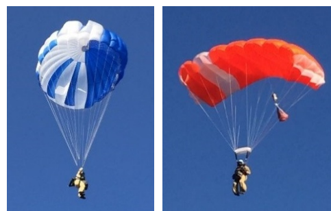
Figure 2. Round (left) and square (right) parachutes.
