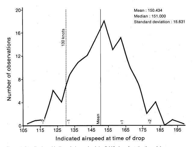
Figure 1. Distribution of indicated airspeeds of the C-119 aircraft at the time of drop.
