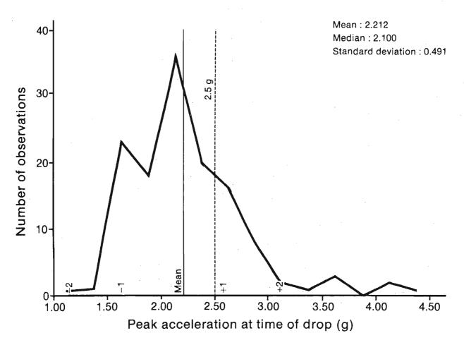
Figure 3. Distribution of peak accelerations at the time of drop from the C-119 aircraft.
