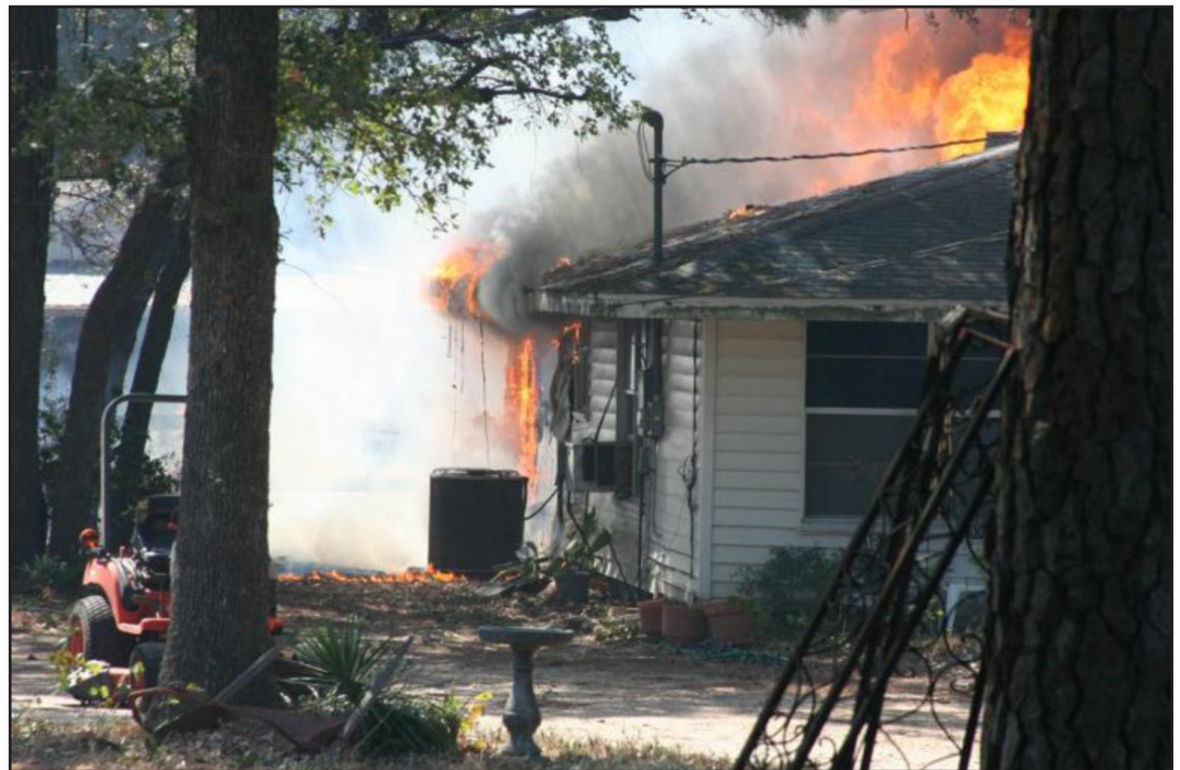
This Bastrop home caught fire after flames crept through surrounding pine needles and bushes until they reached the eaves of the house.
