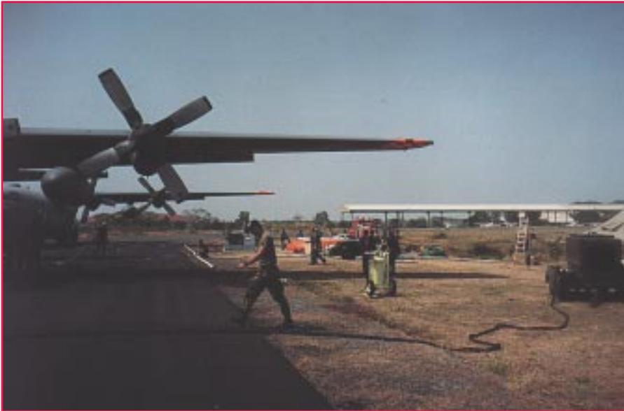
**Figure 2**—The MAFFS portable airbase operating at the Indonesian naval air station in Surabaya. The depression in the ground on the right contains an irrigation ditch that supplied the suppressant (water) dropped by the C-130 MAFFS airtankers throughout operations in eastern Java. Photo: Joe Madar, USDA Forest Service, Fire and Aviation Management, Washington Office, Washington, DC (retired).
