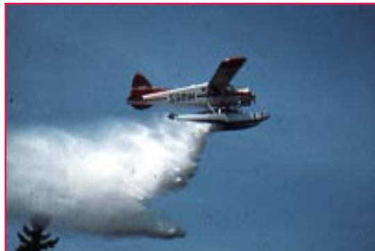
**Figure 1**—A USDA Forest Service DeHavilland Beaver making a water drop. The highly versatile Beaver can also haul cargo and transport personnel. With its floats, it can turn a lake into an instant landing zone. Photo: Minnesota Department of Natural Resources, Grand Rapids, MN, 1997.
