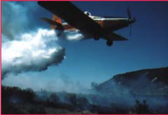
**Figure 3**—A single-engine airtanker (SEAT) working a fire. What the SEAT lacks in payload it makes up in shortened turnaround time. Photo: Minnesota Department of Natural Resources, Grand Rapids, MN, 1997.
