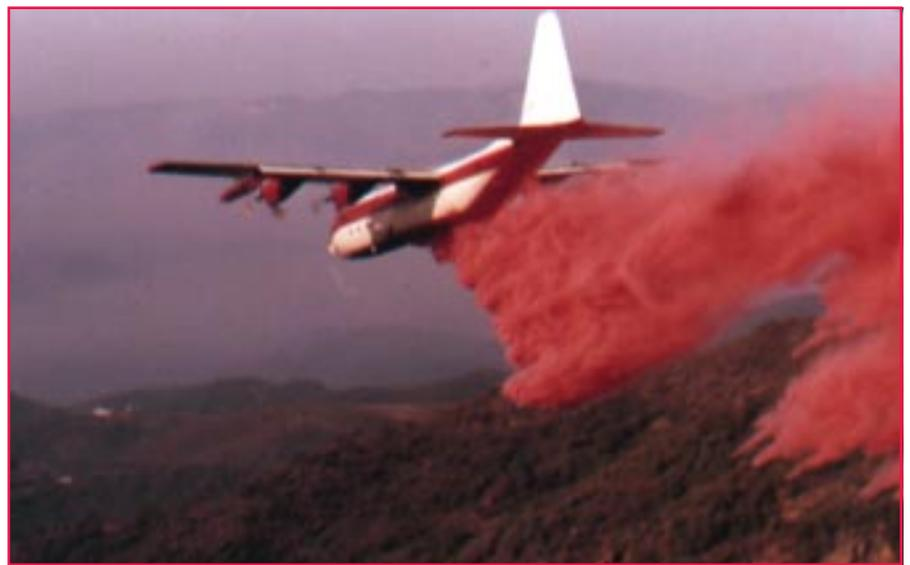
**Figure 1**—A C-130 dropping retardant on a 1994 wildfire in southern California. C-130s are part of the new generation of large airtankers specified in recommendation 2 of the National Airtanker Study, phase 2. Photo: Cecil Stinson, Jr., USDA Forest Service, Shasta-Trinity National Forest, Redding, CA, 1994.
